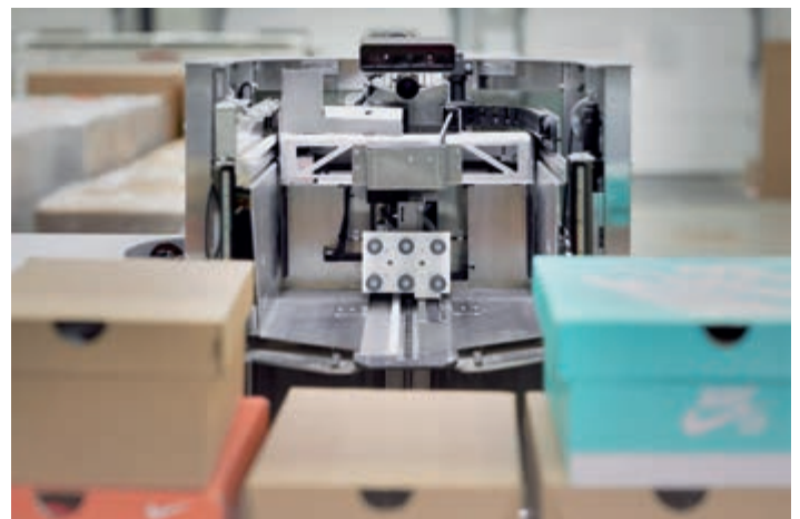
Storage and retrieval is performed by a vacuum gripper arm driven by FAULHABER motors.
