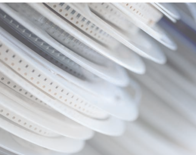
Packaging of tested parts in carrier tape
