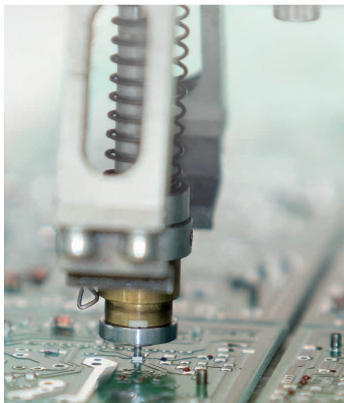
Automatic PCB assembly using the pick & place method
