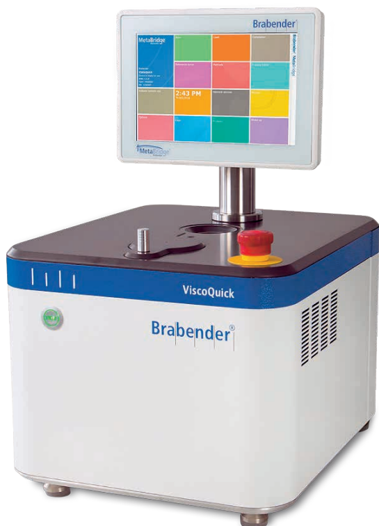
Fast universal measurement device: the ViscoQuick determines the gelatinisation properties of starch, the alpha-amylase activity in flour as well as the absolute viscosity of Newtonian liquids. (Copyright: Brabender)
