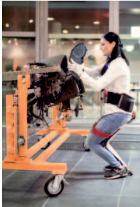
Test run at Audi: The specialist has fetched the speedometer element and is sitting comfortably on the chairless chair from Noonee during installation.
