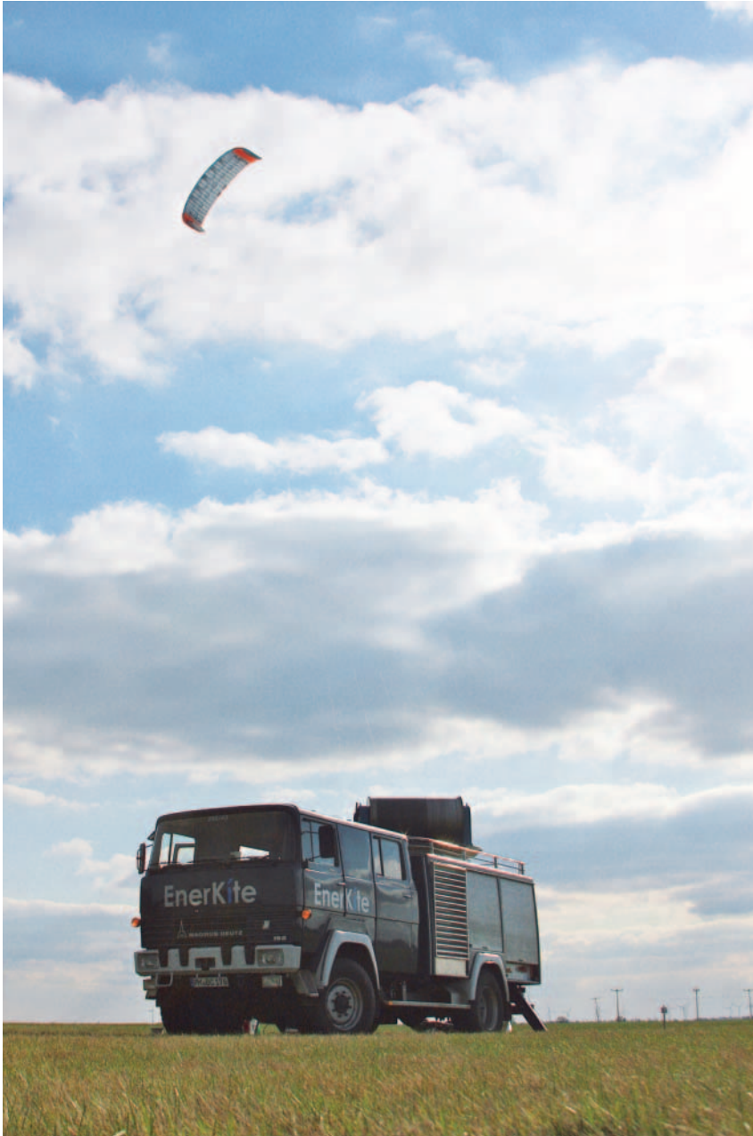
The test turbine with 30 kW and 15 m 2 kite demonstrates the suitability of the concept for practical use
